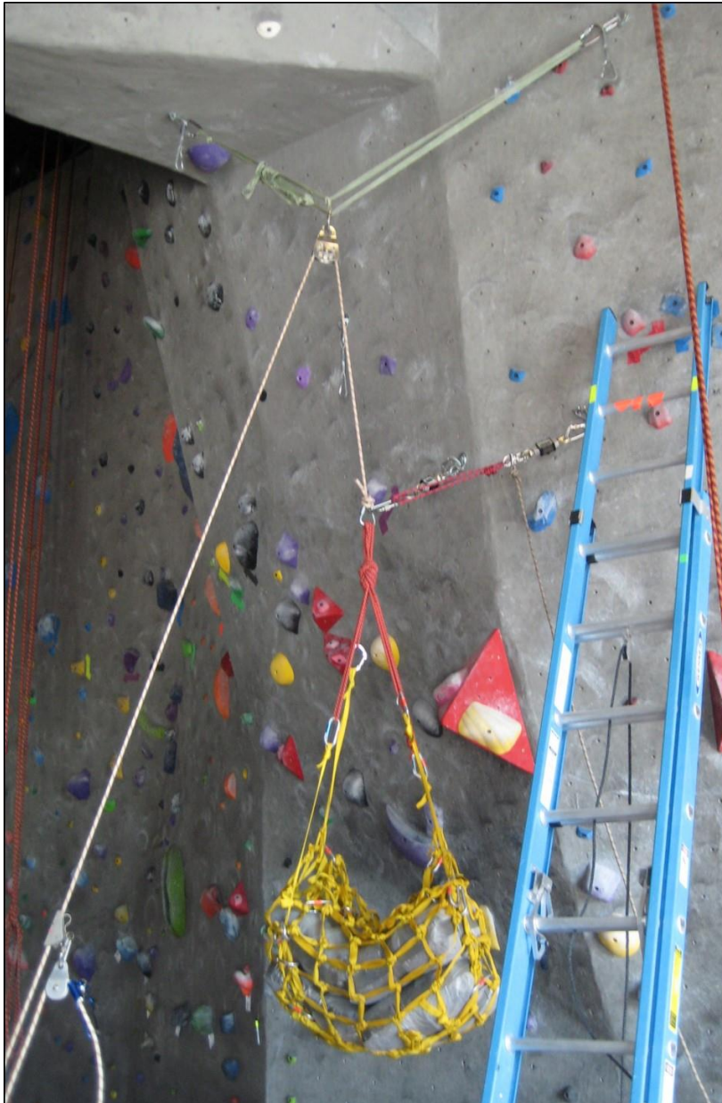
Figure 2: The test mass, four sand bags totaling 120.66kg (266lbs), haul system, and ladder for accessing the bolts and load cells. The load is hanging from the haul system here.
