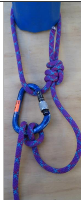
Figure 11: Multidirectional anchor and fixed brake
