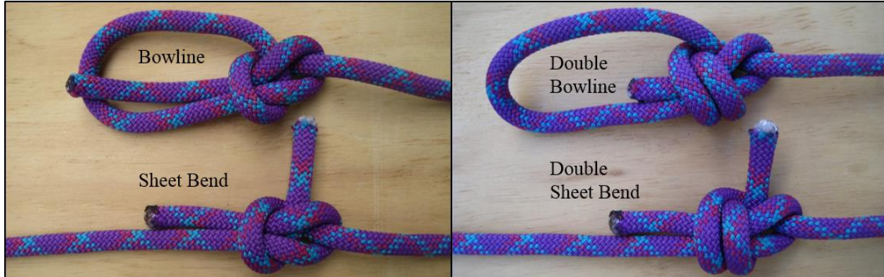
Figure 8: Comparison of bowlines and sheet bends; they are the same series of rope turns.
