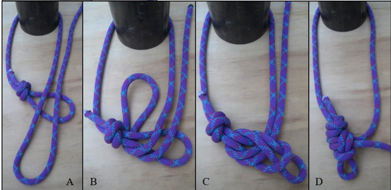
Figure 18: How to tie an Eye Sheet Bend really quickly. With the tail of the rope, tie your chosen backup knot (e.g., overhand or barrel knots) as a slip knot (A). Wrap the rope around the anchor forming a bight (A). Wrap the bight over and under the slip knot loop (B). Finish the knot by passing the bight through the slip knot loop (C). Set and dress the knot (D). Setting will be rapid because the backup knot slips down to the sheet bend when the slip loop is pulled shut. This variation is exceptionally fast, creates a rigging loop pointing down the pitch, and makes it very difficult to incorrectly load the sheet bend pulling the knot apart.
