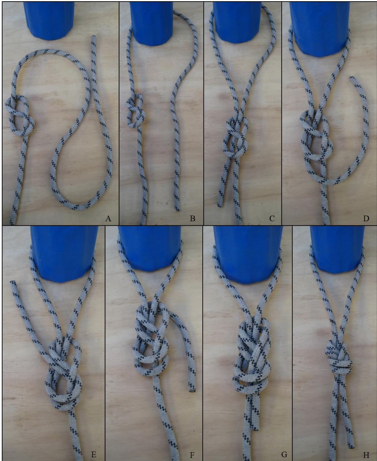
Figure 7: Tying the Figure 8 Follow Through anchor. Tie a figure 8 in the rope (A) and wrap the rope around the anchor (B). Tie a figure 8 follow through starting where the rope left the figure 8 toward the anchor (C-G). Adjust the rope so the remaining tail is not too long, the anchor internal angle is narrow enough, then dress, set, and safety check.
