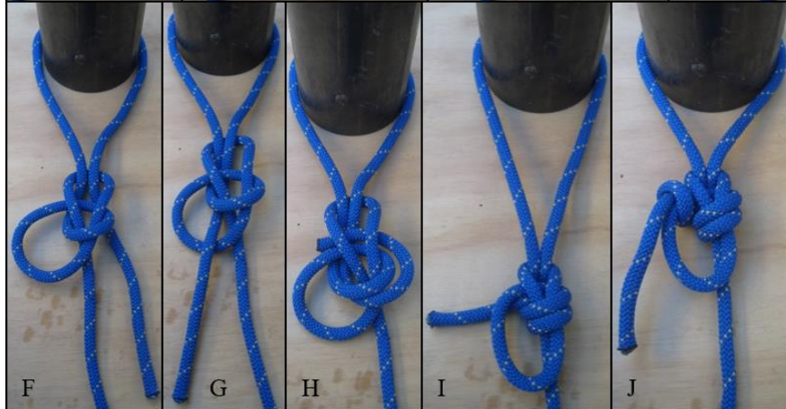
Figure 15: How to tie an Eye Bowline around an anchor. Measure enough rope to go around the anchor (A), add some extra rope enough to backup the knot (B), tie a bowline (C-E), thread the tail through the knot (F-H), set and dress (I), and add a backup knot (J).
