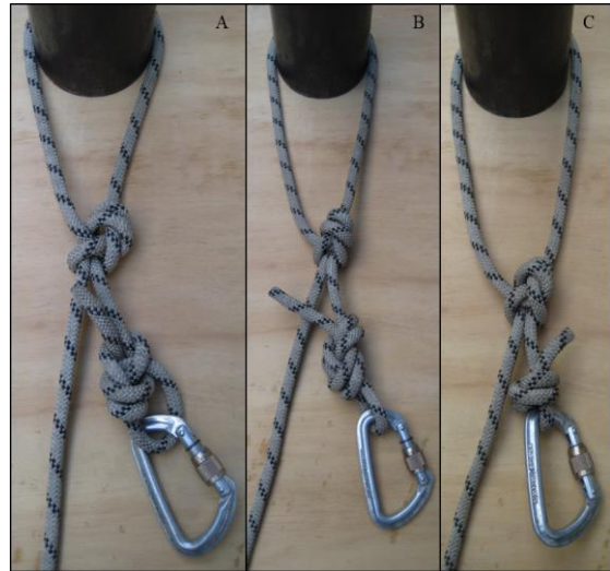
Figure 14: Knot tail modifications, A) Bowline, B) Figure 8, and C) Scaffold knot.
