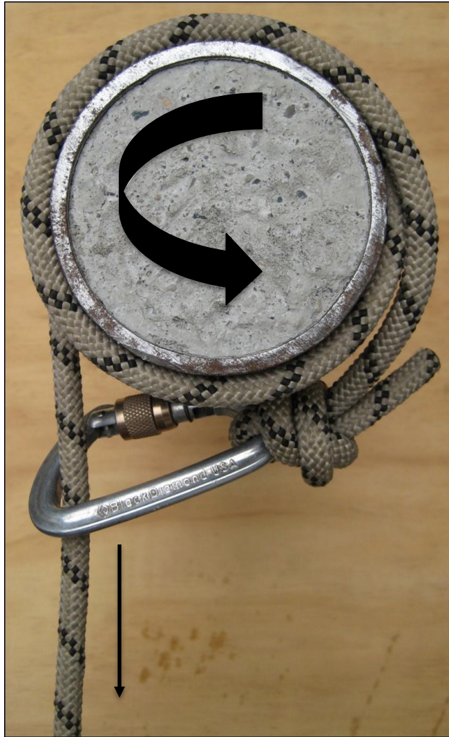
Figure 3: Force applied to an HST and the resulting force on the anchor.
