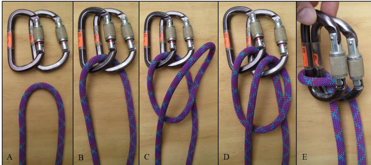
Figure 2: How to tie the Garda Hitch. A) Two similar “D” shaped carabiners oriented with gates down, B) Clip the rope through both carabiners, C) Form a loop of rope on one side of the two carbiners, D) Clip the loop of rope into the far carabiner, E) Set and dress the Garda Hitch ensuring the two carabiners are snug against each other.
