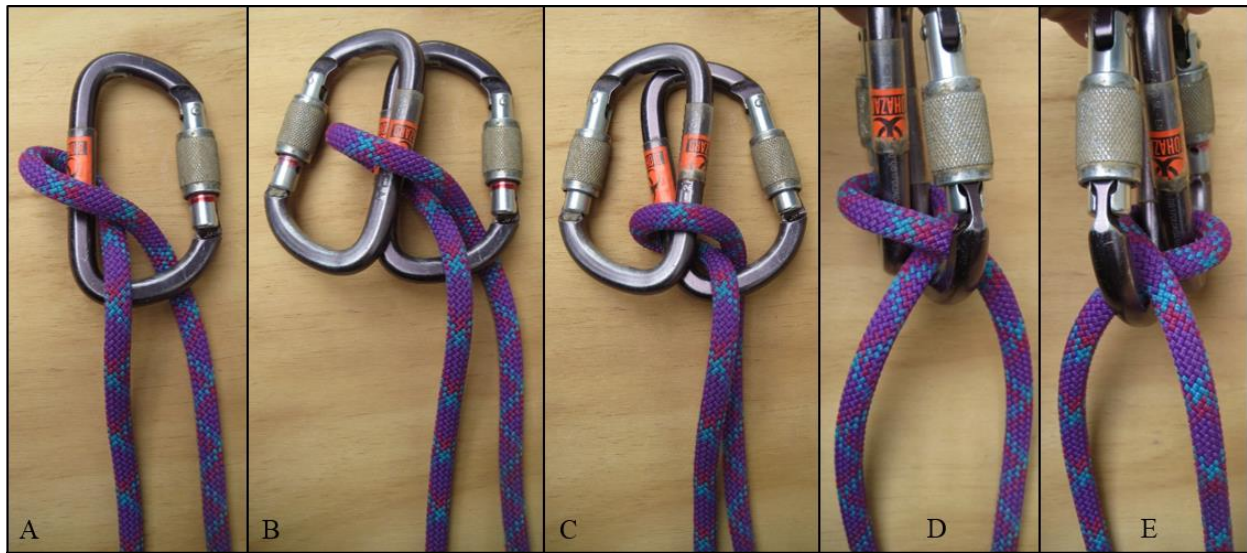
Figure 7: How to tie the Heart Brake. A) Clip a carabiner through the X in a loop of rope, B) Clip a second carabiner through the loop of rope with the carabiner gate facing the opposite direction. The carabiner should be clipped on the same side of the first carabiner as the bottom strand of rope comes out. C) The two carabiners should be clipped onto an anchor so both lay tight against each other. D) The final hitch should look like this panel. E) If the hitch looks like this, you should move the second carabiner to the other side of the first carabiner so it looks like panel D.
