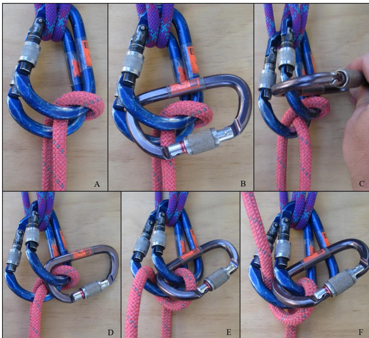
Figure 5: Converting the Garda Hitch to a lower. A) Start by tying a Garda Hitch, B) Connect a third carabiner to the carabiner on the slack side of the hitch, C) The third carabiner can be used as a lever to torque the first two carabiners apart, D) Move the third carabiner between the two strands of rope, E) Collapse the Garda Hitch so that the rope no longer pinches against itself, F) If you need less friction, move the control strand toward the anchor, which will reduce the friction in the hitch.
