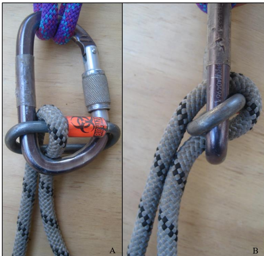
Figure 10: Construction and orientation of the Mallion System. A) The correct orientation of the mallion so it will not unscrew when the rope runs over it and with the rope against the carabiner spine. B) A side view of the Mallion System to illustrate the path the rope takes around the hardware.
