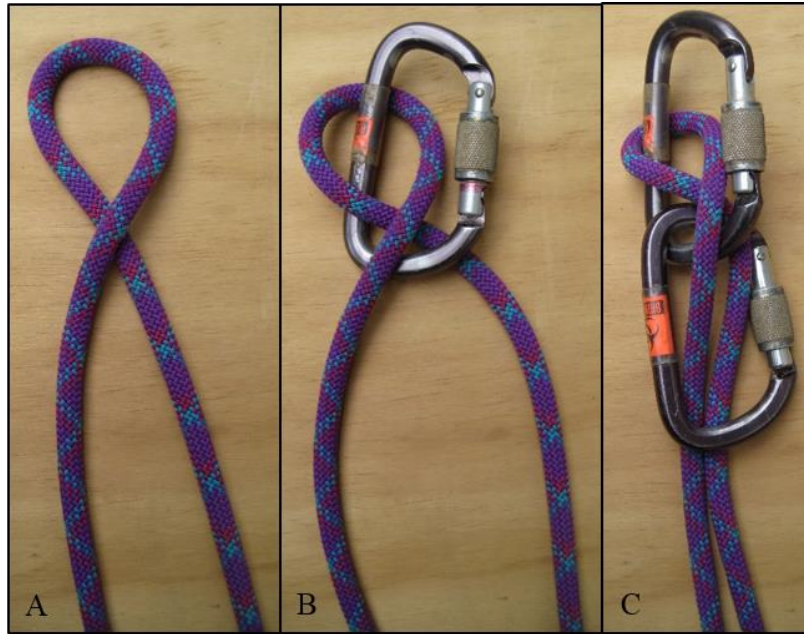
Figure 6: How to tie the Lorenzi Hitch. A) Form a loop in the rope, B) Clip the X created by the loop with the carabiner, C) Clip a second carabiner between the rope and the first carabiner's spine, and capture the two strands of rope hanging below the hitch.
