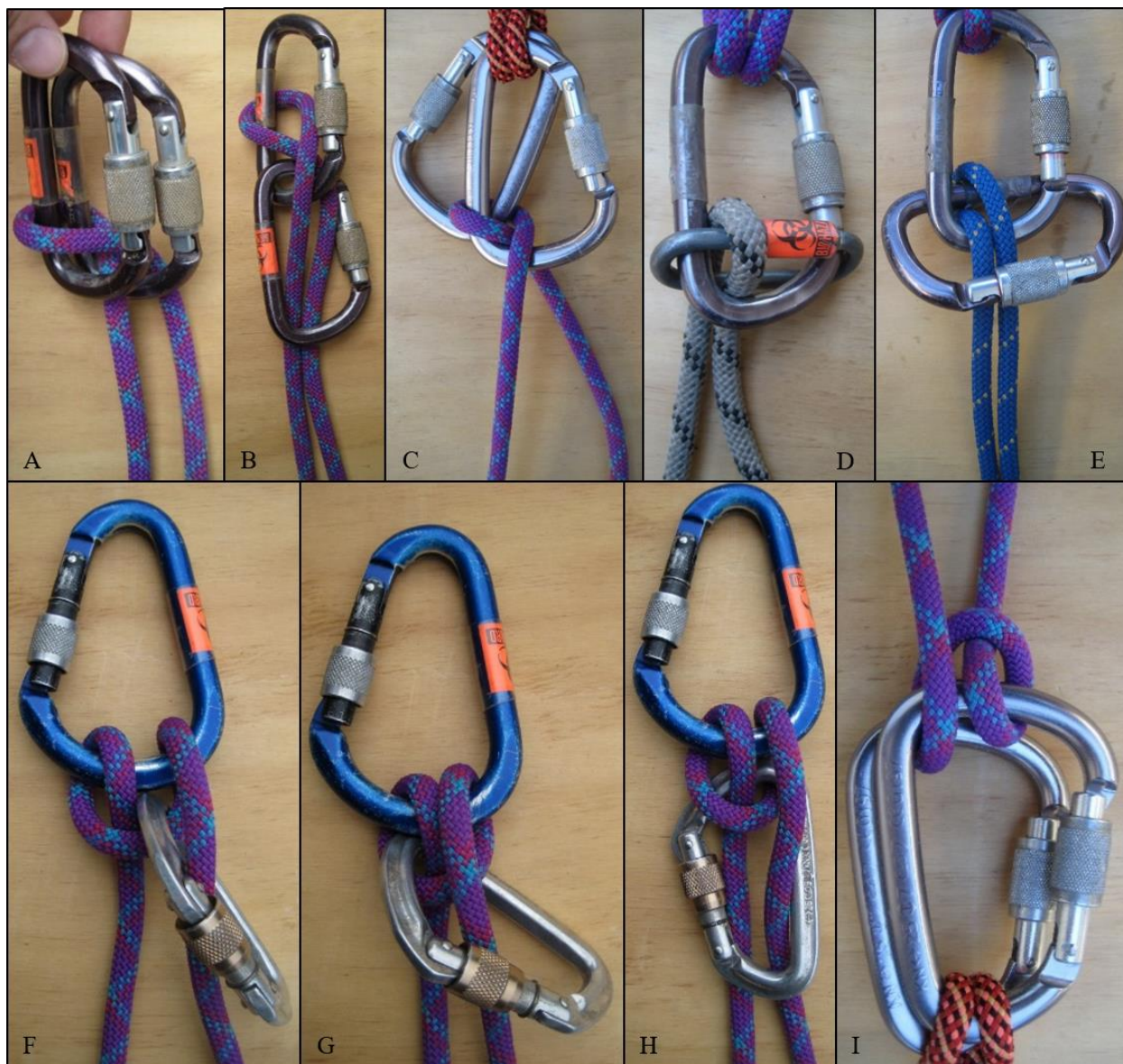
Figure 1: All nine hitches described here. A) The Garda Hitch, B) The Lorenzi Hitch, C) The Heart Brake, D) The Mallion System, E) The Carabiner System, and four one way Münter Hitches F) Münter Hitch variation #1, G) Münter Hitch variation #2, H) Münter Hitch variation #3, and I) The Remy Hitch.
