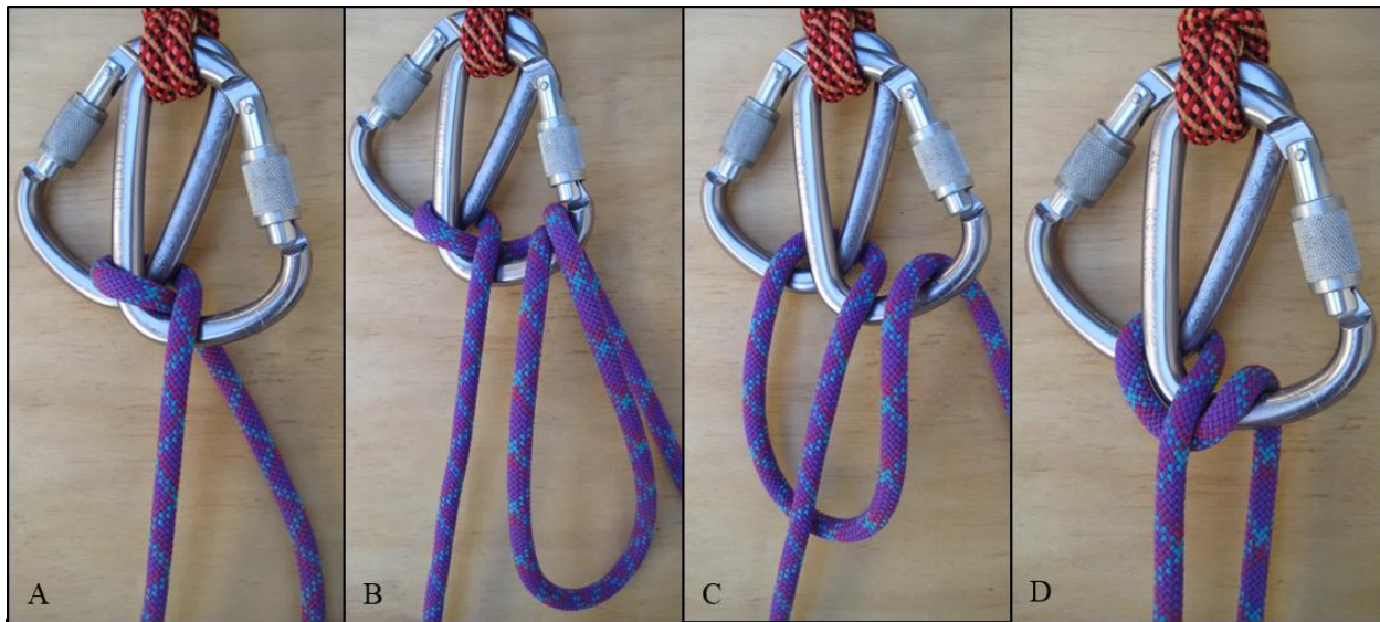
Figure 9: How to unlock the Heart Brake. A) Tie a Heart Brake, B) Pass a bight of the slack end through the carabiner, C) Pull down hard to pop the rope out from under itself, D) Dress the Heart Brake, which forms a hitch close to the Münter Hitch. Lower the load as needed. To lock up the hitch simply pull hard on the control side which will reform the hitch.
